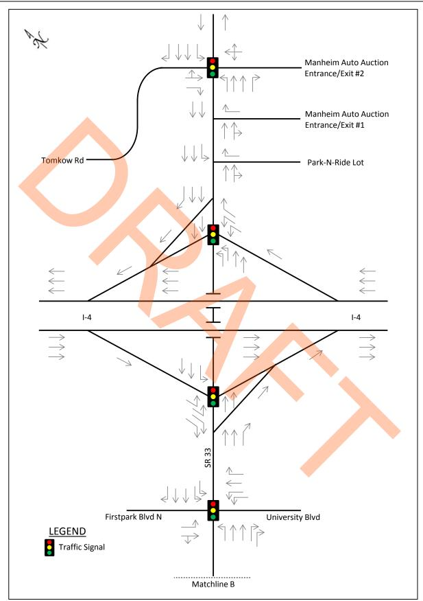
FIGURE 6-2: DESIGN YEAR (2036) RECOMMENDED INTERCHANGE/INTERSECTION GEOMETRY – BUILD ALTERNATIVE
