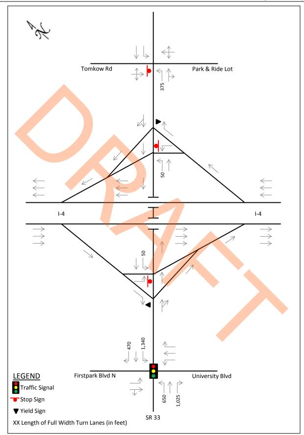
FIGURE 2-2: EXISTING YEAR (2012) INTERCHANGE/INTERSECTION GEOMETRY
