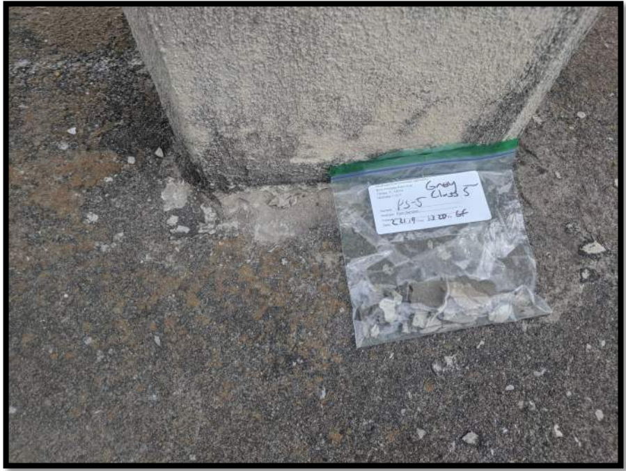
Photograph 51 View of Metals Based Coating Sample PS-5 (Gray Class 5).
