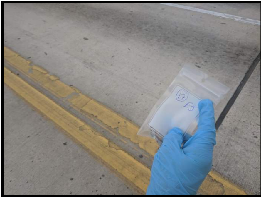
Photograph 17 View of Asbestos Homogeneous Area 6 – Expansion Joints - Roadway (Sample Location 16).
