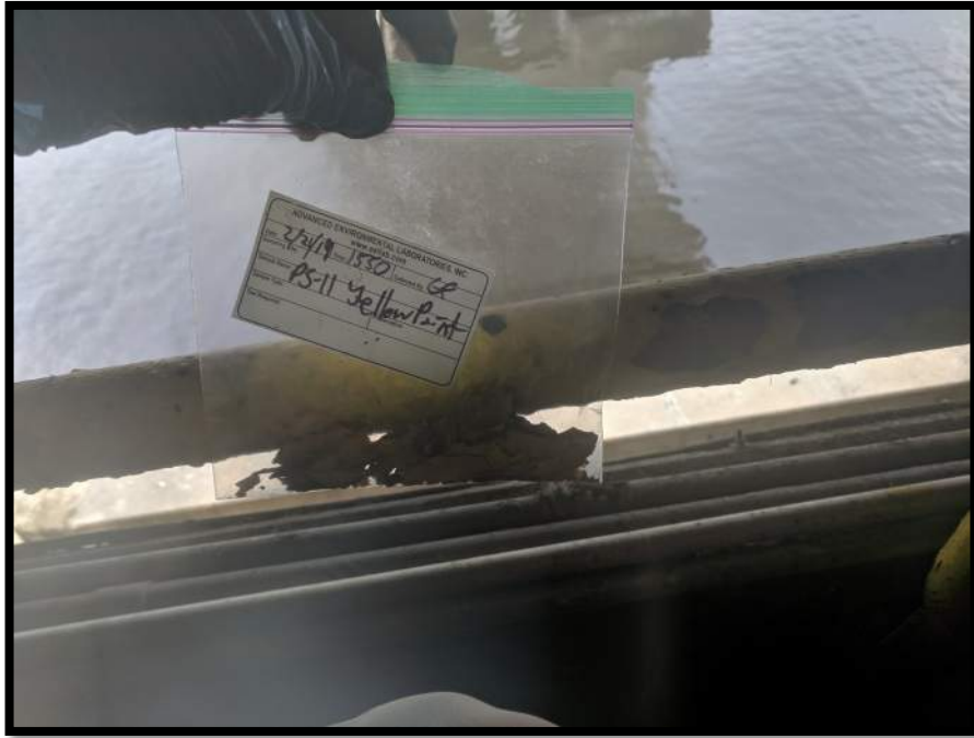
Photograph 57 View of Metals Based Coating Sample PS-11 (Yellow Paint).
