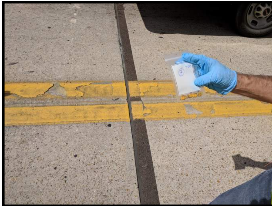
Photograph 8 View of Asbestos Homogeneous Area 3 – Yellow Lane Paint – Roadway Deck (Sample Location 7).
