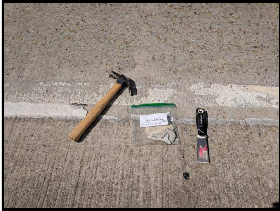
Photograph 47 View of Metals Based Coating Sample PS-1 (White Lane Paint).
