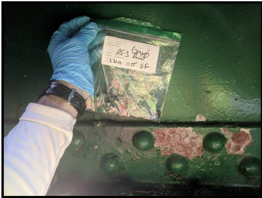
Photograph 49 View of Metals Based Coating Sample PS-3 (Green Paint).
