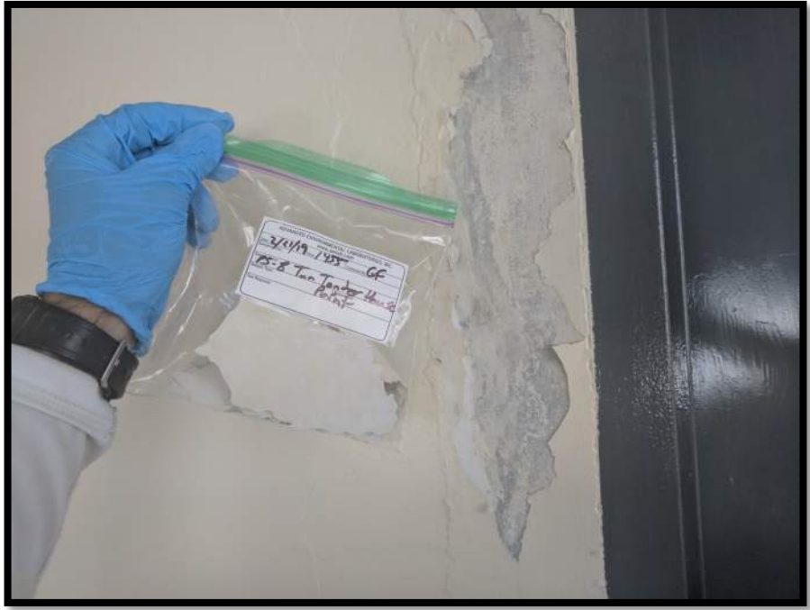
Photograph 54 View of Metals Based Coating Sample PS-8 (Tan Tender House Paint).
