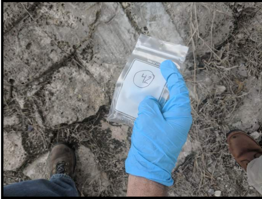
Photograph 43 View of Asbestos Homogeneous Area 14 – Rip Rap - Embankments (Sample Location 42).
