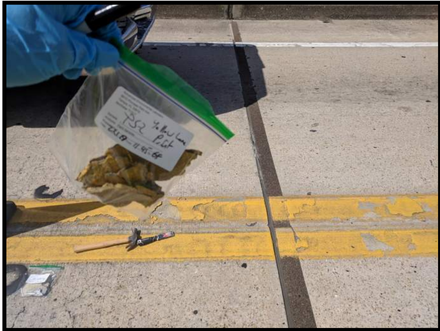
Photograph 48 View of Metals Based Coating Sample PS-2 (Yellow Lane Paint).
