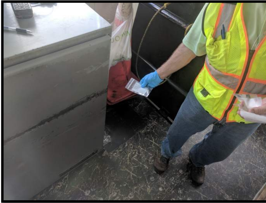
Photograph 21 View of Asbestos Homogeneous Area 7 – 12"x12" Floor Tile and Adhesive Mastic (Bottom Layer) – Tender House (Sample Location 20).
