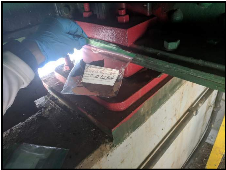
Photograph 56 View of Metals Based Coating Sample PS-10 (Red Paint).
