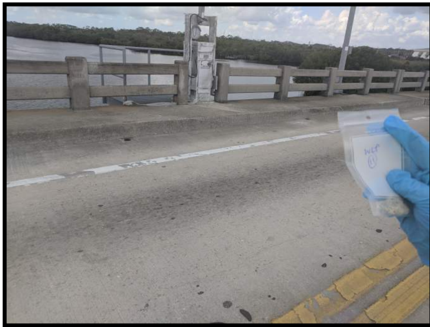
Photograph 12 View of Asbestos Homogeneous Area 4 – White Lane Paint – Roadway Deck (Sample Location 11).
