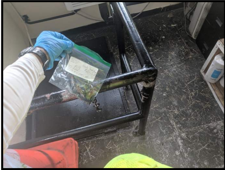
Photograph 55 View of Metals Based Coating Sample PS-9 (Black Tender House Paint).
