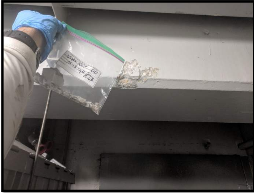
Photograph 59 View of Metals Based Coating Sample PS-13 (Light Gray Paint).
