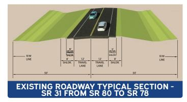
Within the project limits, SR 31 is a two-lane roadway with 12-foot lanes and 4 to 8-foot paved shoulders. Stormwater runoff is collected in roadside ditches, with ultimate discharge to the Caloosahatchee River. The posted speed limit is 40 miles per hour. To address traffic growth, FDOT is proposing to widen the existing roadway.
