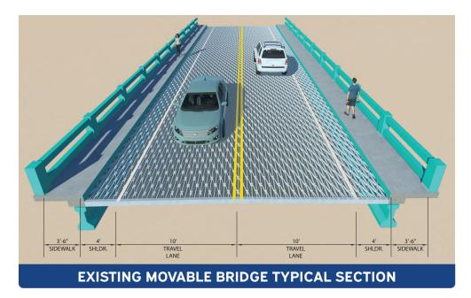
The Wilson Pigott Bridge currently has two 10-foot lanes, 4-foot shoulders, and 3.5-foot sidewalks on both sides with no separation from motor vehicles. The existing vertical clearance over the channel is 21 feet.
