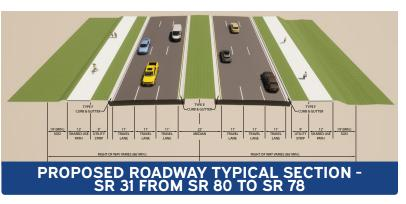
The proposed improvement would consist of widening the twolane roadway to six lanes and, as shown in the proposed typical section, includes three 11-foot lanes in each direction, curb and gutter, a 22-foot raised median, and 12-foot shared use paths on both sides to accommodate pedestrians and bicyclists. The project would require the acquisition of additional right of way for roadway improvements and drainage. The proposed posted speed limit is 45 miles per hour.
