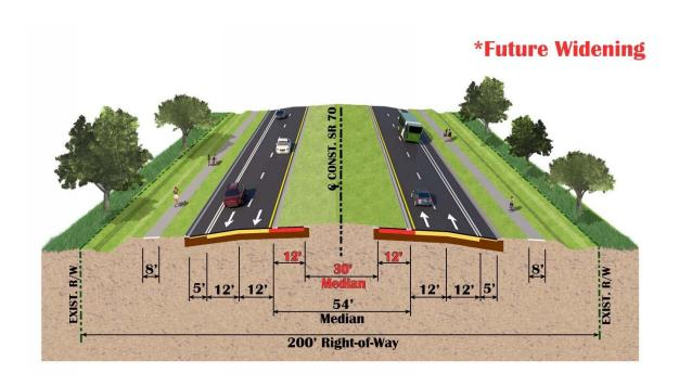
Figure 2-5 Segment C Proposed Typical Roadway Section
