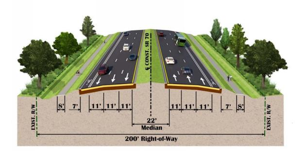
Figure 2-3 Segment A Proposed Typical Roadway Section
