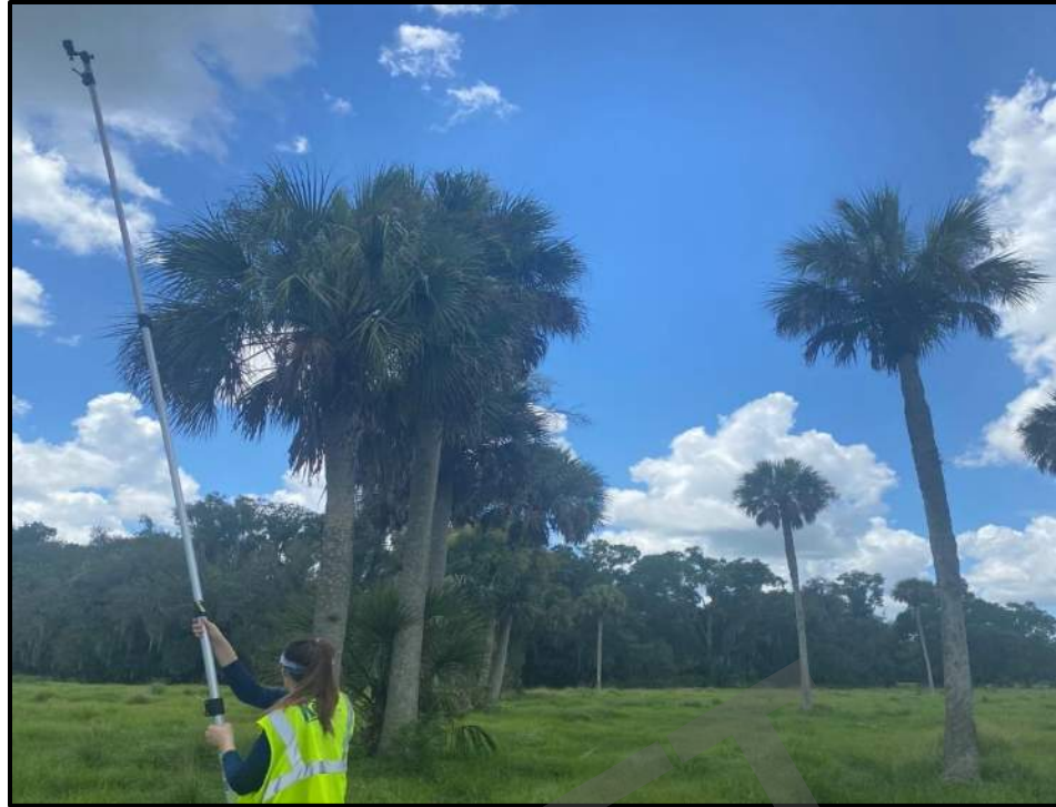
Photo 1. Photograph of the extension pole with attached camera for viewing out of reach potential roosting structures.
