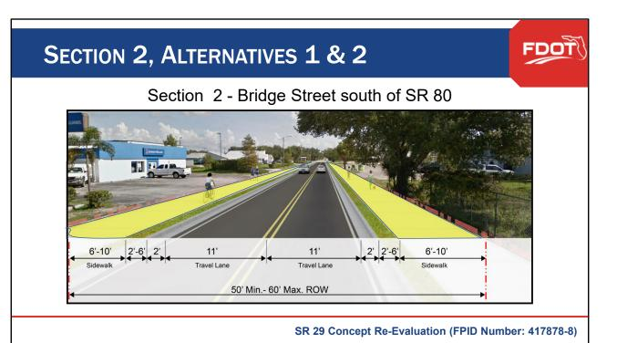
Section 2 Bridge Street south of SR 80 currently has two 12-ft travel lanes, a center two-way turn lane, and 6ft paved sidewalk on both sides of the roadway. Businesses along the corridor provide parking within their parcels.
