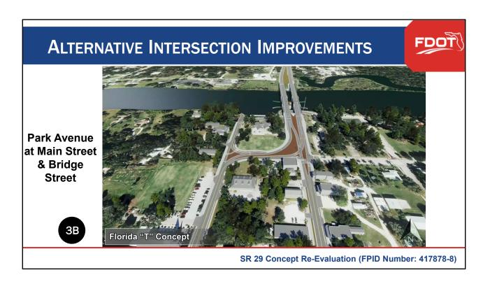
The Florida T intersection features a continuous northbound travel lane and a continuous southbound bypass lane to Main Street. This concept will include pedestrian push button-activated signals working with the traffic signal. In addition, the Florida "T" will not impact Barron Park, provides a traffic-calming and potential gateway feature, and capacity well beyond 2040.
