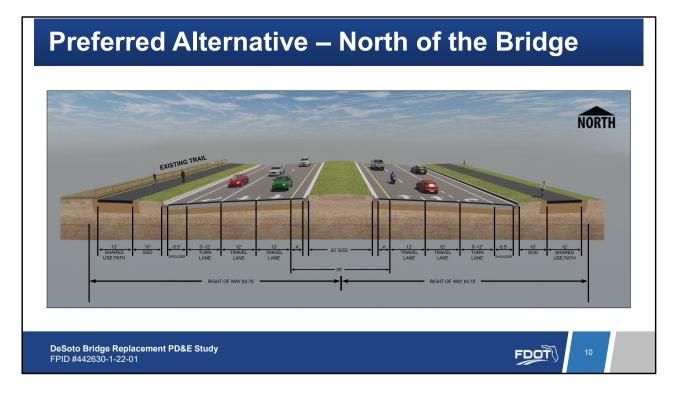
North of the bridge the typical section includes two 12-foot travel lanes in each direction and a 12-foot shared use path on both sides of the road. In the southbound direction there is one westbound turn lane. The northbound direction includes one eastbound and one westbound turn lane. The typical section also includes a seven-foot concrete traffic separator and a swale on the west side of the road for drainage.
