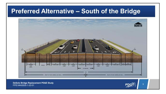
South of the Bridge the typical section includes two 12-foot travel lanes and one 12-foot turn lane in each direction, a shared use path on the west side of the road and a 6-to-8-foot sidewalk on the east side of the roadway. The typical section also includes 10-foot inside shoulders and a swale on the west side of the road for drainage.
