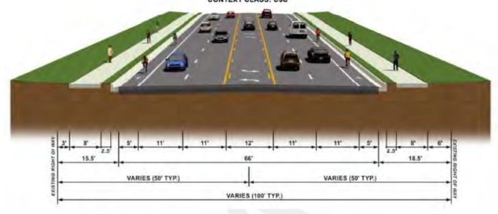
Figure 1-4. Typical Section of the proposed Hurricane Pass Bridge Improvements
