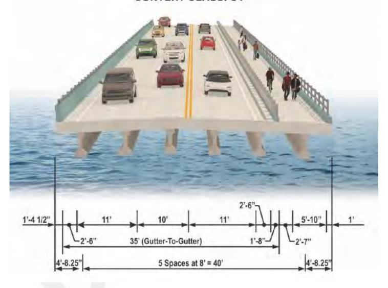
Figure 1-3. Typical Section of the SR 865 (San Carlos Boulevard) improvements from Main Street north to Hurricane Pass Bridge
