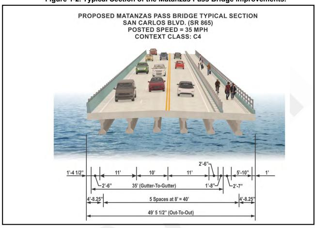
Figure 1-2. Typical Section of the Matanzas Pass Bridge improvements.
