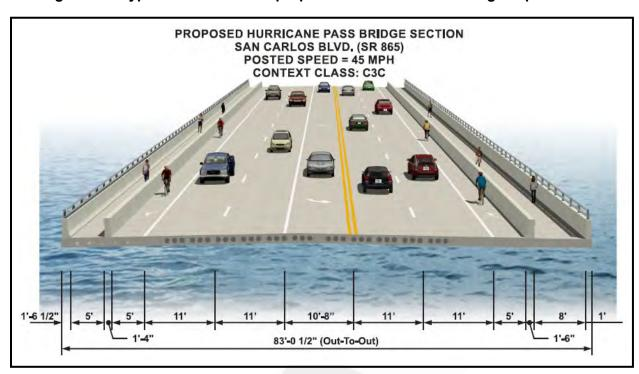
Figure 1-4. Typical Section of the proposed Hurricane Pass Bridge improvements.
