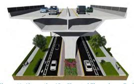
Figure 40: Alternative AB - Elevated Throughway Typical Section - Between the Manatee River & Manatee Avenue
