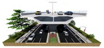
Figure 41: Alternative AB - Elevated Throughway Typical Section - North of the Manatee River
