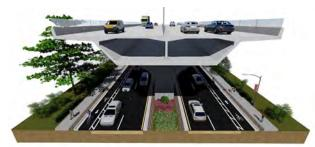
Figure 43: Alternative B - Elevated Throughway Typical Section: South of Manatee Avenue
