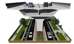
Elevated Throughway Typical Section: Two Lanes at Local Level
