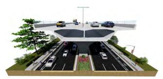
Elevated Throughway Typical Section: Six Lanes at Local Level
