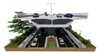
Figure 39: Alternative AB - Elevated Throughway Typical Section - South of Manatee Avenue
