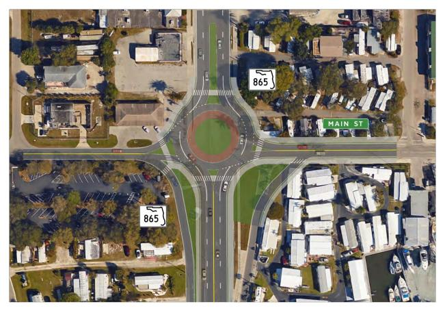
Figure 8 Roundabout Concept at SR 865 and Buttonwood Drive/Prescott Street
