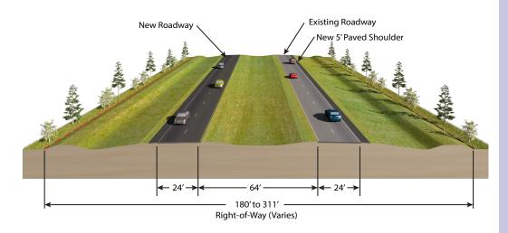
FDOT's contractor, Ajax Paving Industries of Florida, is constructing 12-foot wide travel lanes in each direction with a 64-foot grassed median. Additional work includes repaving the current lanes on SR 80 and constructing ten new bridges. Three bridges will require full demolition and removal of the existing bridges to construct the new ones.
