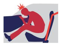
An **unrestrained occupant** continues to travel forward until rapidly striking the steering column, windshield, or other part of the vehicle, causing serious injury.
