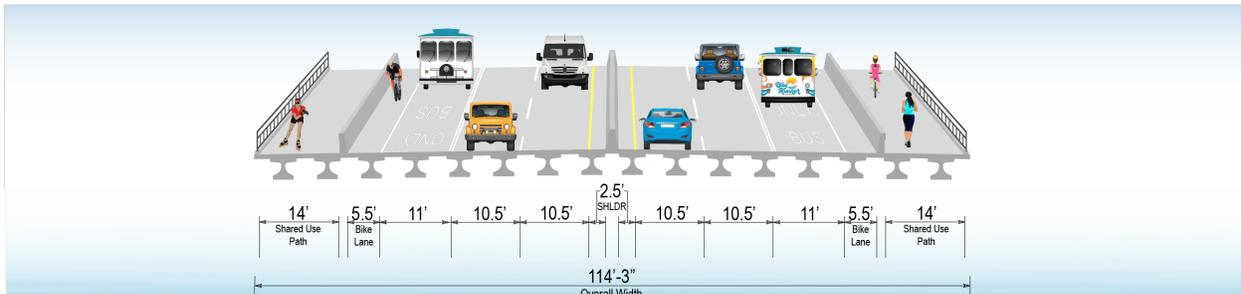
The new bridge will transition to a curb and gutter roadway typical section that includes two 10.5-ft wide travel lanes, a dedicated 11-ft transit lane, and 5-ft bike lane in each direction, separated by a median with Type E curb and gutter. This section of roadway also includes a 10-ft shared-use path on both sides of the roadway that connects to the bridge, shown on **Figure 7-2**. The design speed is 40 mph with a posted and target speed of 35 mph.
