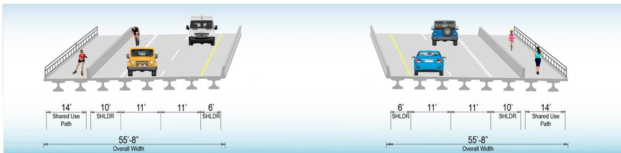
5.4.1.3 Step 3: Initial Horizontal and Vertical Geometry5.4.1.3.1 Single Bridge Alternative
