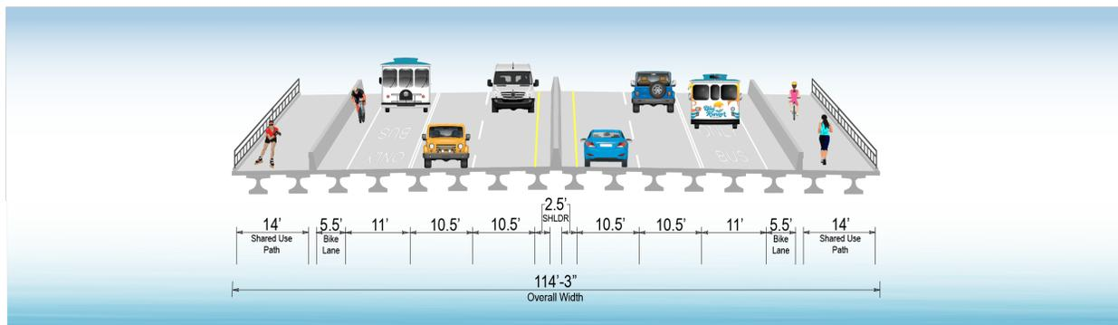
The new bridge will transition to a curb and gutter roadway typical section that includes two 10.5-ft wide travel lanes, a dedicated 11-ft transit lane, and a 5-ft bike lane in each direction, separated by a median with Type E curb and gutter. This section of roadway also includes a 10-ft shared-use path on both sides of the roadway that connects to the bridge, shown on **Figure 1-3**. The design speed is 40 mph with a posted and target speed of 35 mph.
