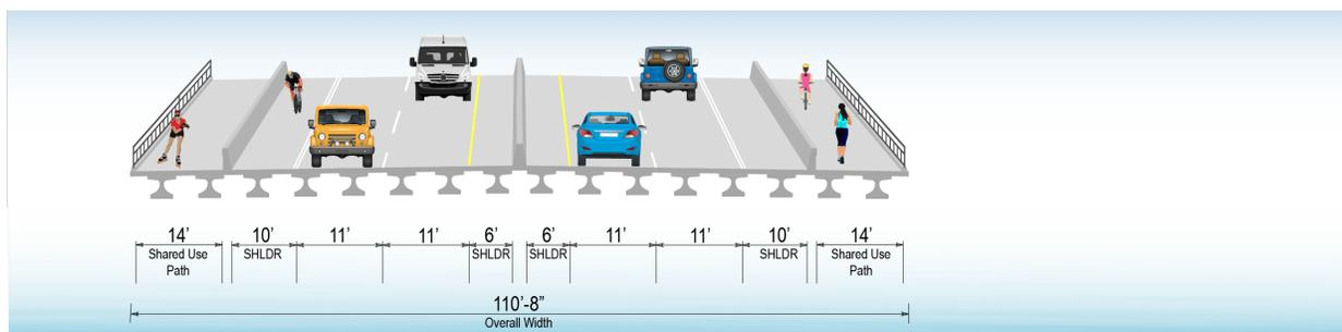
The twin bridge typical section includes two 11-ft wide travel lanes with 6-ft inside and 10-ft outside shoulders, and 14-ft shared use paths in each direction. The clear space between the twin bridges is 48-ft-4-in. The total width of each bridge is 55 ft 8-in, shown on **Figure 5-3**.
