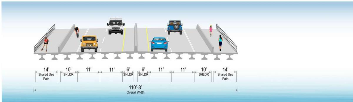
The single bridge alternative will replace the two existing bridges with a single structure for all lanes of travel. The travel lanes on the new bridge will be the same 11-foot width as on the existing bridges. 10-foot outside shoulders will accommodate bicyclists, and a 14' shared use path would be added to each side of the bridge.
