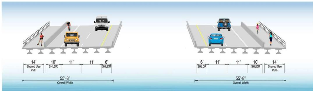
The twin bridges alternative will replace the two existing bridges with individual bridges for each direction of travel. The travel lanes on the new bridges will be the same 11-foot width as on the existing bridges. 10-foot outside shoulders will accommodate bicyclists, and a 14' shared use path would be added to the outside of each bridge.
