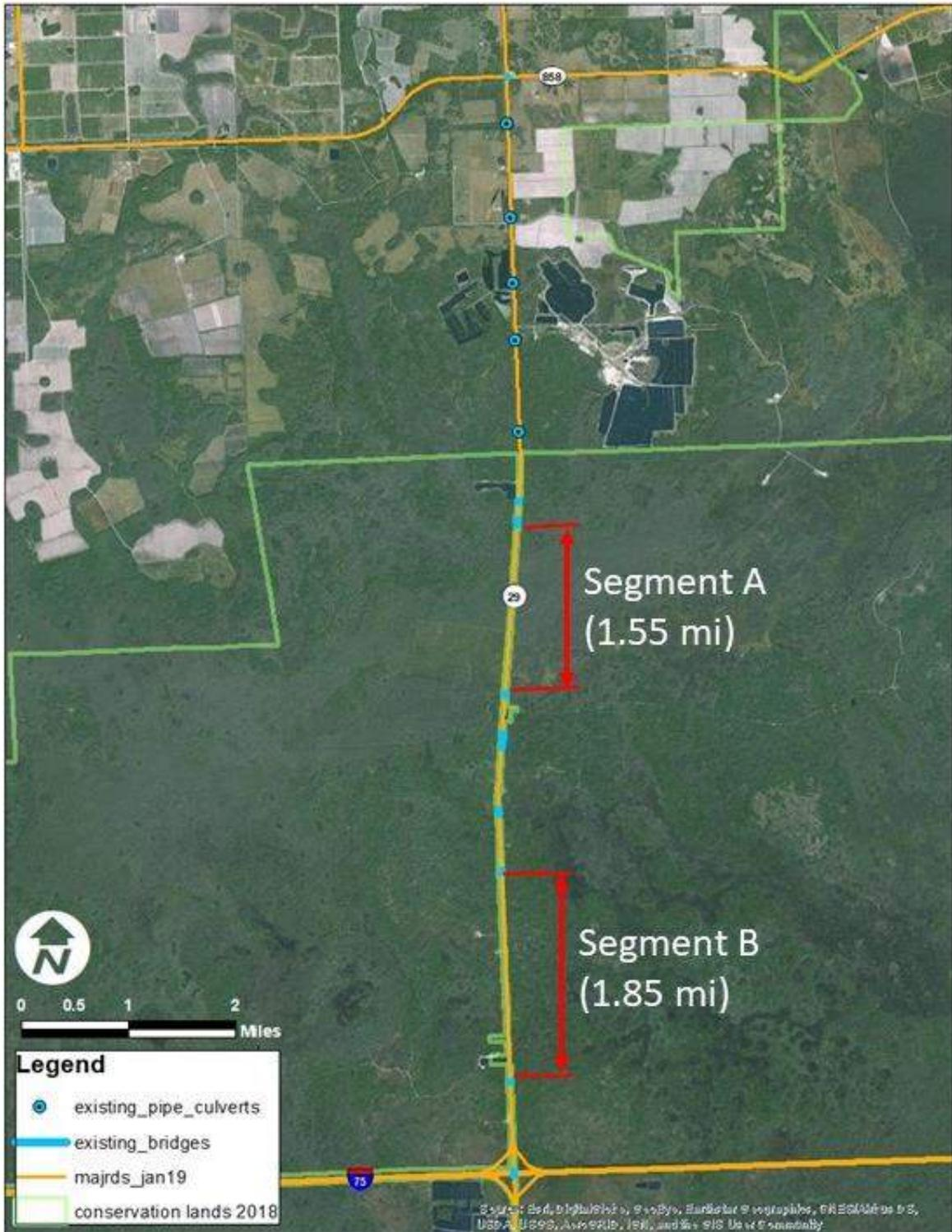
**Figure 8. Extended gaps between wildlife crossing structures in the south section of the SR 29 project area. These segments should be considered for installation of smaller culvert crossings for wildlife.**
