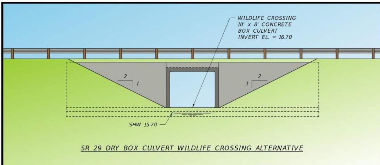
Figure 17 SR 29 Alternative 2 Elevation View
