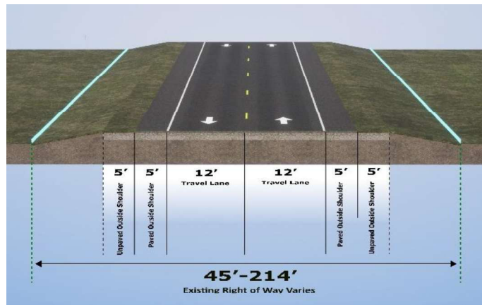
Figure 1-2: Existing Typical Section
