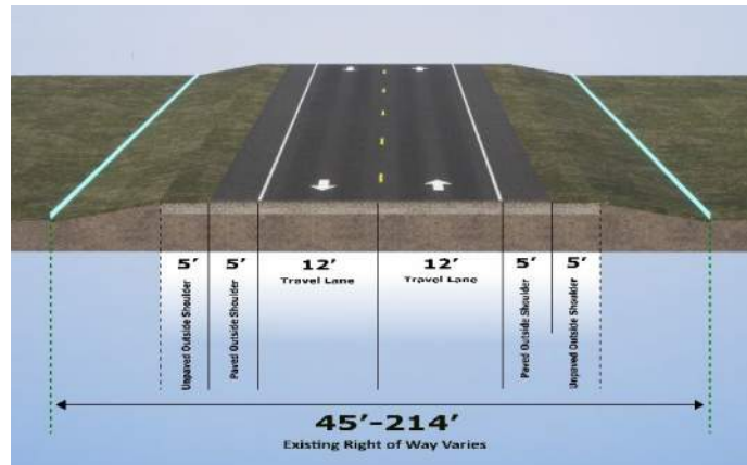
Figure 1-2: Existing Typical Section
