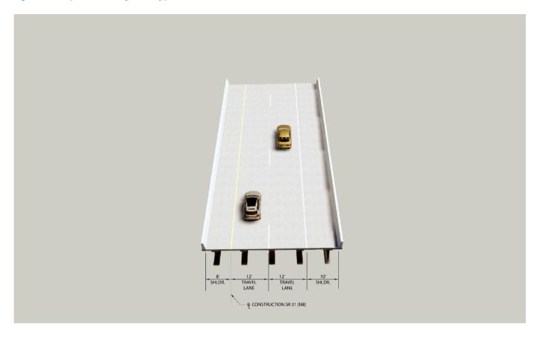
Figure 7. Proposed SB Flyover Typical Section
