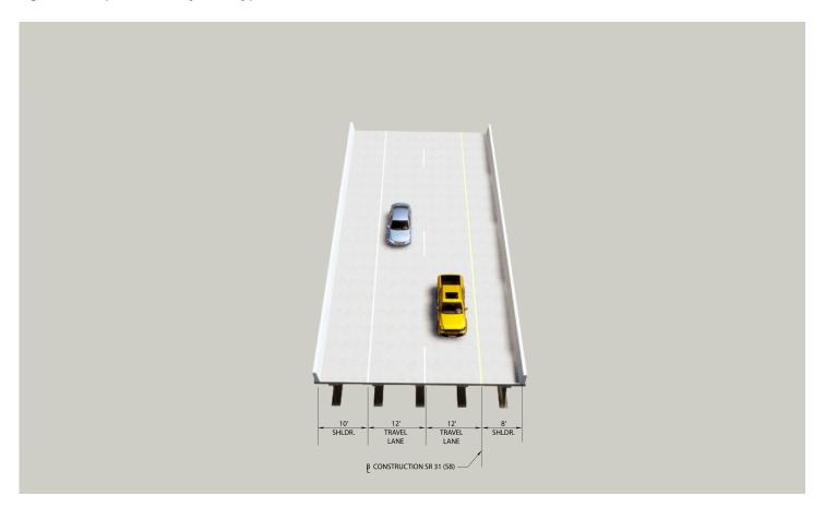
Figure 8. Proposed SR 80 Roadway Typical Section (West of SR 31)
