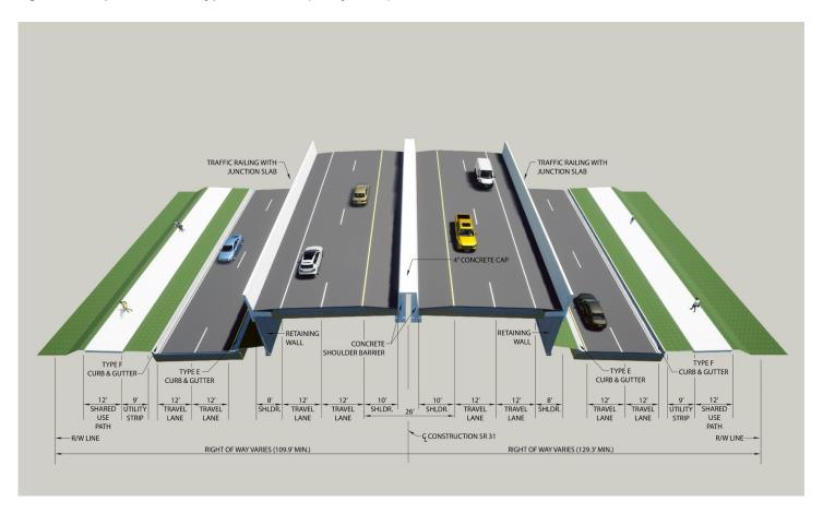
Figure 6. Proposed NB Flyover Typical Section
