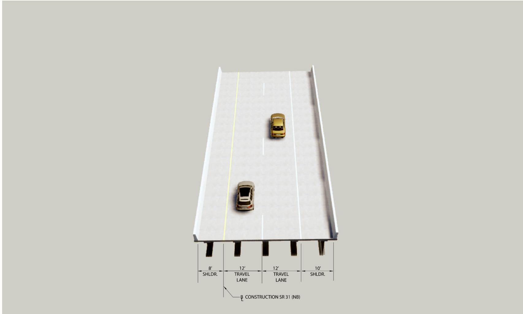
Figure 1-7. Proposed SB Flyover Typical Section
