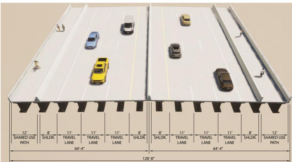
**HIGH-LEVEL FIXED BRIDGE (ALTERNATIVES 1A/1B) TYPICAL SECTION - SR 31 AT CALOOSAHATCHEE RIVER**
