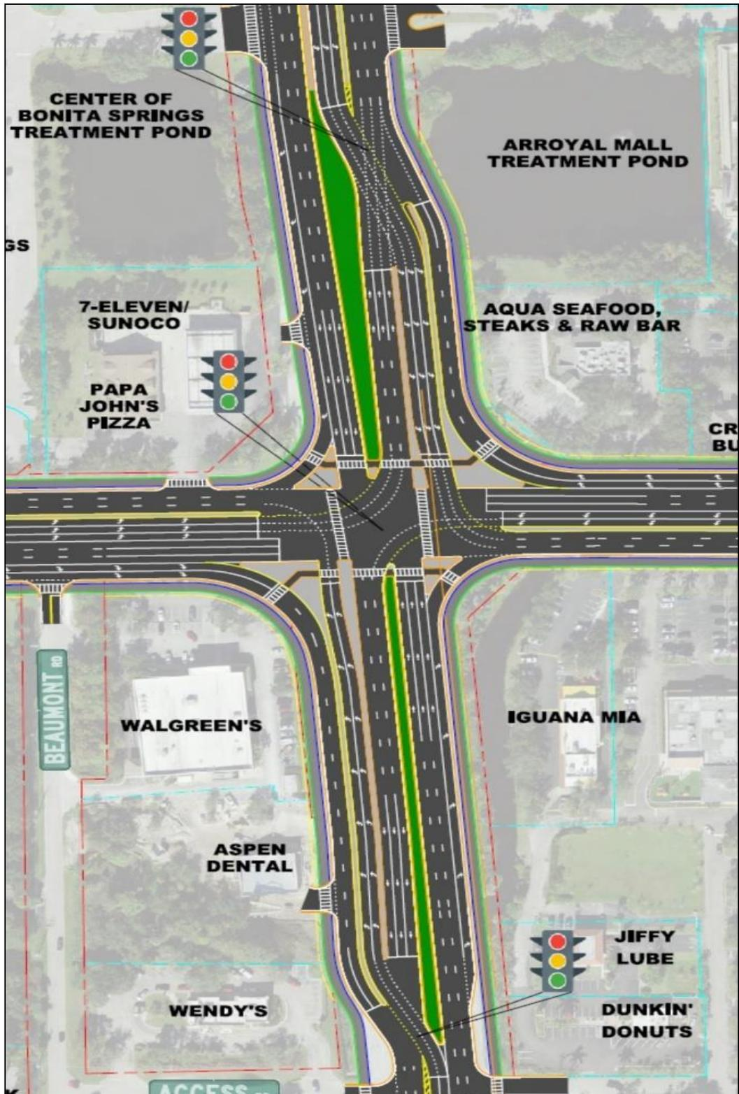
Figure 3: Partial Displaced Left Turn Alternative
