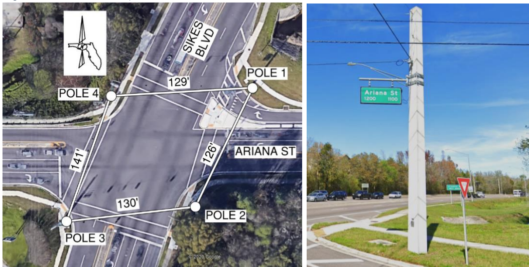
Left image: aerial showing strain pole locations and span lengths at the intersection of Sikes Blvd. and Ariana St. Right image: Pole 1.
