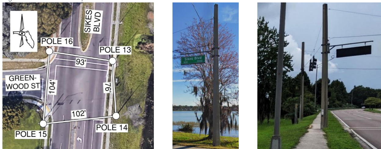
Left image: aerial showing strain pole locations and span lengths at the intersection of Sikes Blvd. and Greenwood St. Middle image: Pole 14. Right image: a view of Pole 13 (foreground) and Pole 14
