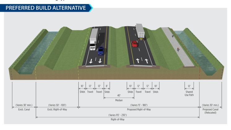
The Preferred Build Alternative typical section includes 12-foot travel lanes, 10-foot (5-foot paved) outside shoulders, a 10-foot (5-foot paved) inside shoulder for eastbound travel lanes, an 8-foot (4-foot paved) inside shoulder for the westbound travel lanes, and a 12-foot shared use path on the south side of the roadway.
