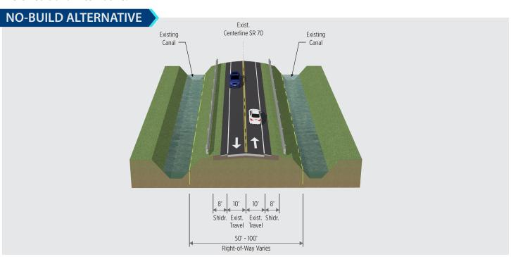
The No-Build Alternative remains a valid option and will continue to be evaluated until the completion of this study. The No-Build Alternative assumes no improvements to SR 70 through the year 2045, except for routine maintenance. The existing typical section includes two 10-foot travel lanes and 8-foot shoulders.
