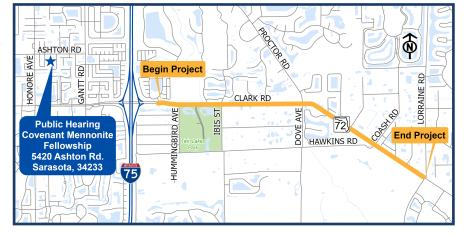
including commercial traffic. SR 72 from east of I-75 to Lorraine Road is currently a two-lane undivided roadway with intermittent right-turn and left-turn lanes. Improvements may include widening to a four-lane divided roadway as well as bicycle and pedestrian accommodations such as a shared-use path.
