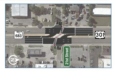
Improvements at the 21st Street intersection also includes adding a restricted crossing U-turn (RCUT) and Pedestrian Hybrid Beacons (PHB) on mast arm assemblies. Additional improvements include replacing and adding signal heads at the intersections of 12th Street, 17th Street, and Dr. Martin Luther King Jr. Way.
