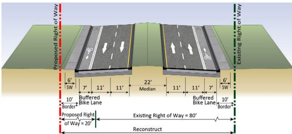
Figure 3-8 New Market Road Typical Section from SR 29 to North of Airport Access (Central Alternative #1 Revised)
