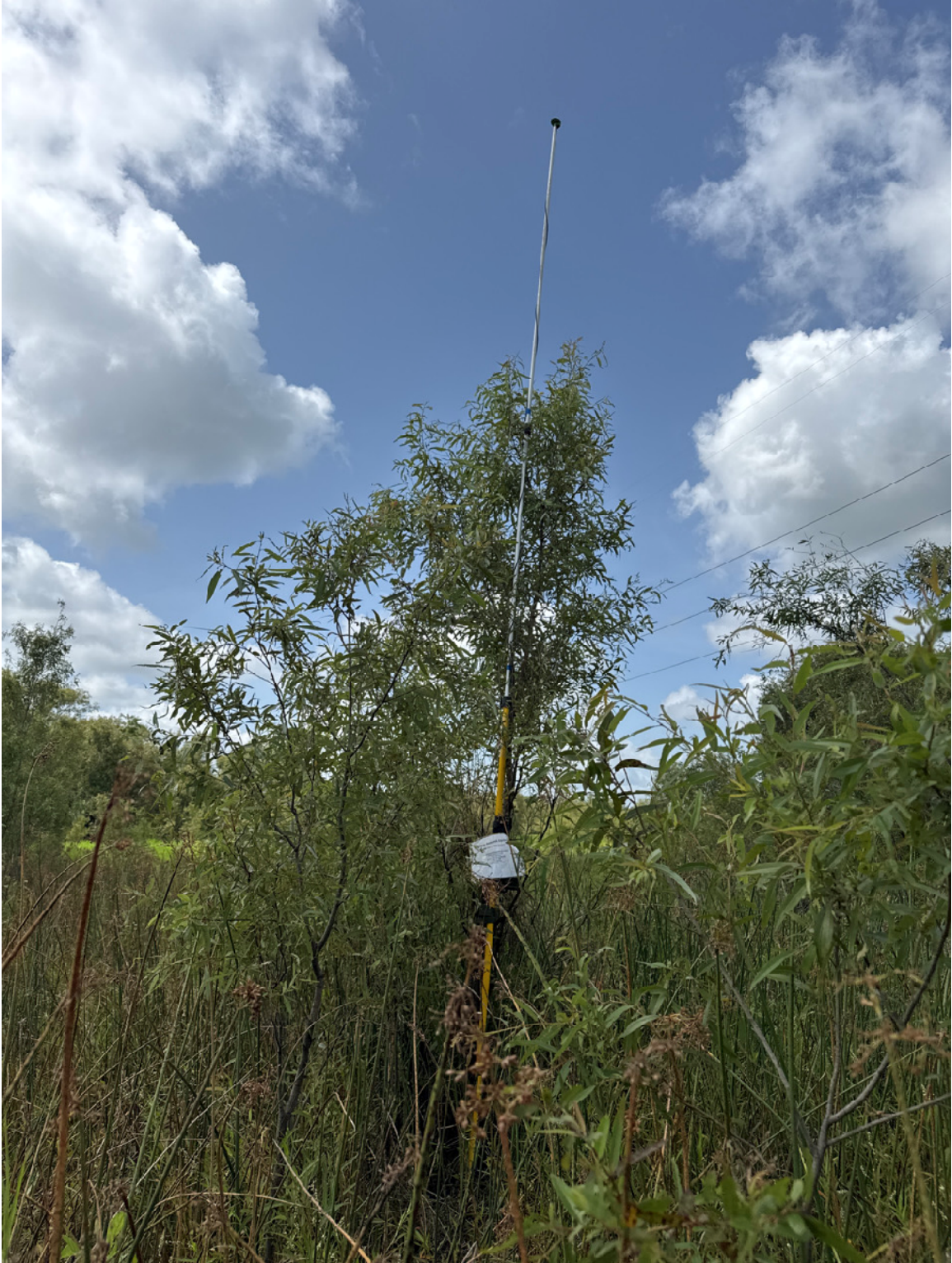
Photograph 3. Photograph looking southwest at Detector 3 with microphone deployment height of 10 meters – Wildlife Acoustics Song Meter SM4BAT FS Ultrasonic Recorder with SMM U2 Ultrasonic Mic.
