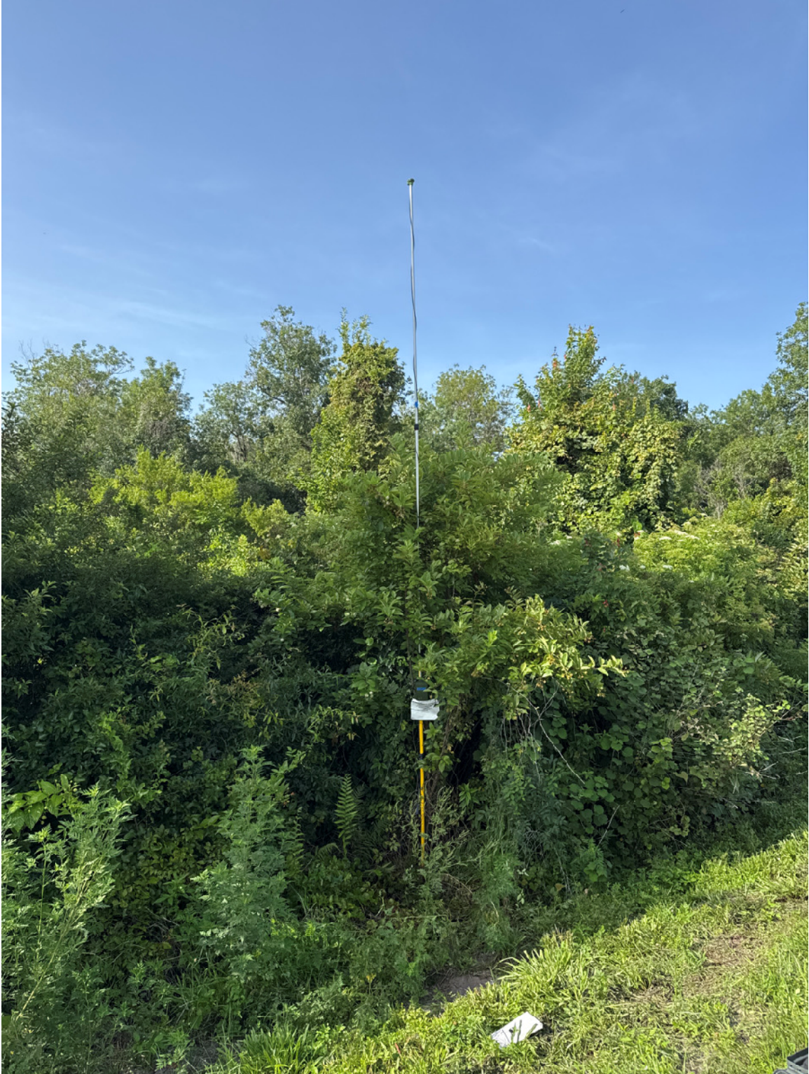
Photograph 1. Photograph looking south at Detector 1 with microphone deployment height of 7 meters – Wildlife Acoustics Song Meter SM4BAT FS Ultrasonic Recorder with SMM U2 Ultrasonic Mic.
