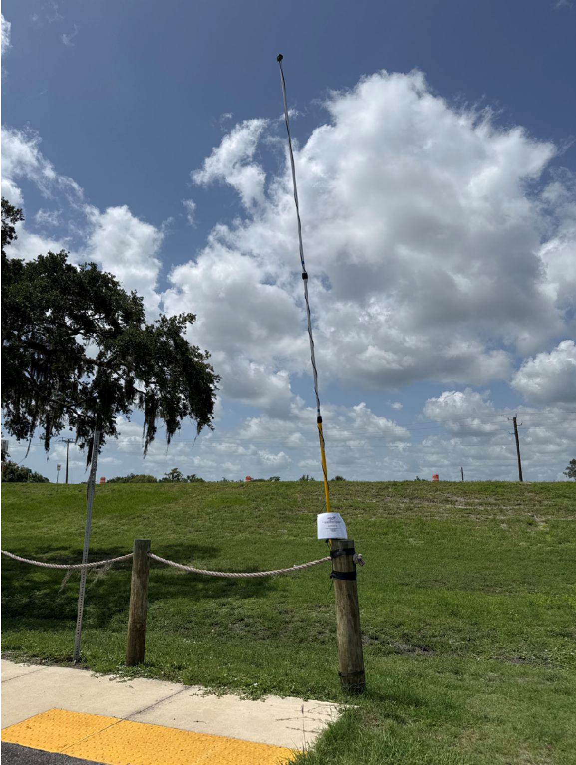
Photograph 4. Photograph looking south at Detector 4 with microphone deployment height of 6 meters – Wildlife Acoustics Song Meter SM4BAT FS Ultrasonic Recorder with SMM U2 Ultrasonic Mic.
