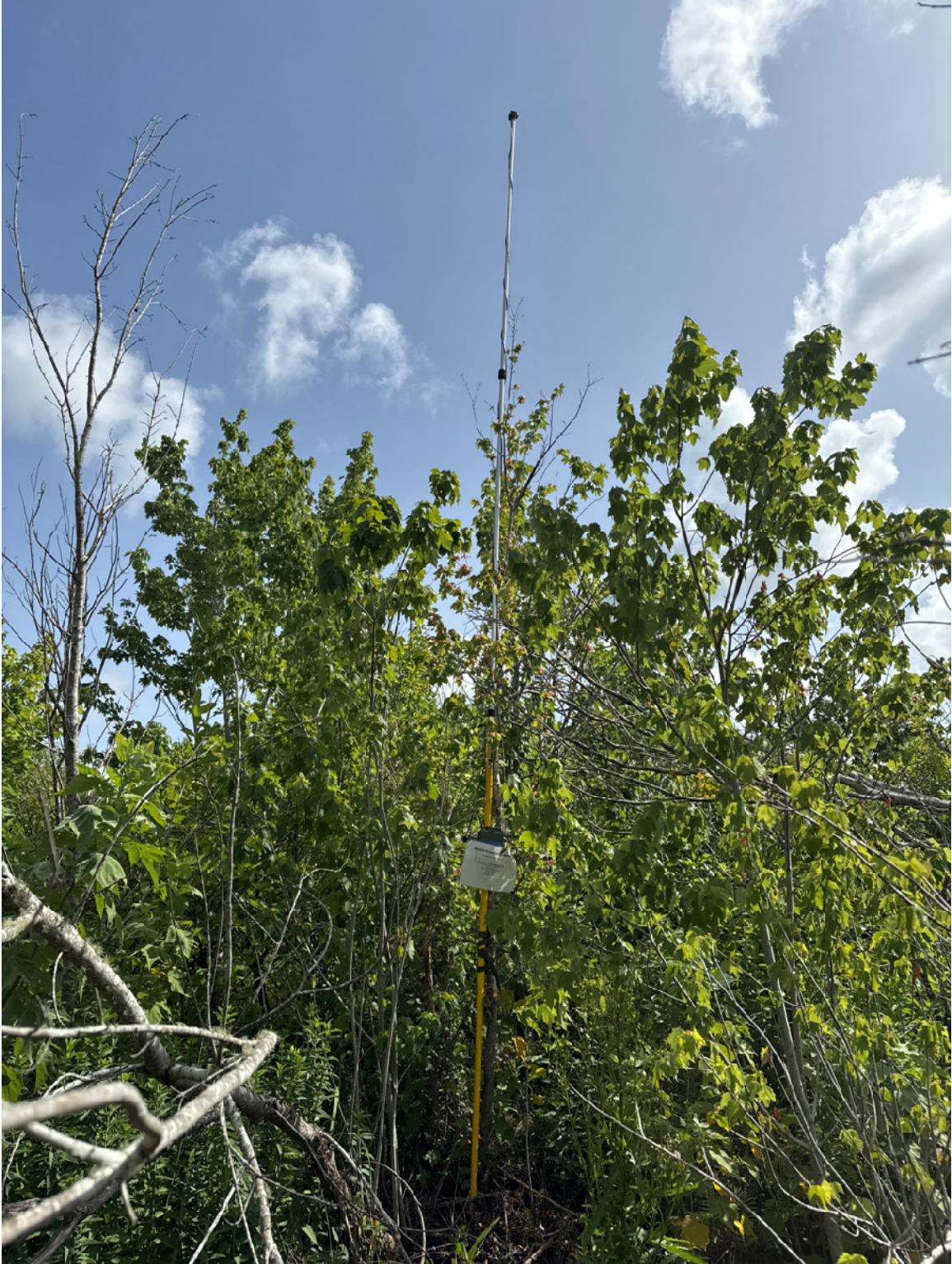
Photograph 2. Photograph looking north at Detector 2 with microphone deployment height of 7 meters – Wildlife Acoustics Song Meter SM4BAT FS Ultrasonic Recorder with SMM U2 Ultrasonic Mic.
