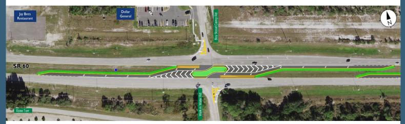
The improvement will consist of reconstructing the median opening to a directional median island. A left-turn lane will be constructed at the median opening to the east of the intersection, to accommodate rerouted U-turning traffic. U-turn aprons will also be constructed at the median openings to the east and west to accommodate U-turning large trucks. Construction of these improvements is planned to begin in Spring 2023 and be completed by the end of 2023.
