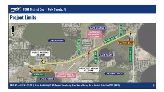
The resurfacing project extends from just west of Jersey Rd to just west of State Road 555, also known as US 17. Within the project corridor, State Road 600 is a four lane, rural road lacking sidewalk access. It contains interspersed center turn lanes and median openings and has a posted speed limit of 55 miles per hour.
