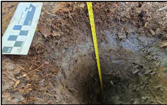
Photo 26. Stratigraphy within the tree island in the northeast portion of Pond 7A, facing north. Note similar stratigraphy is found in the scrub hammock environment of Pond 8A.
