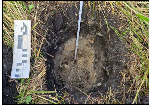
Photo 25. General stratigraphy example within seasonally wet pasture environments, facing north, terminated early due to compacted clay.
