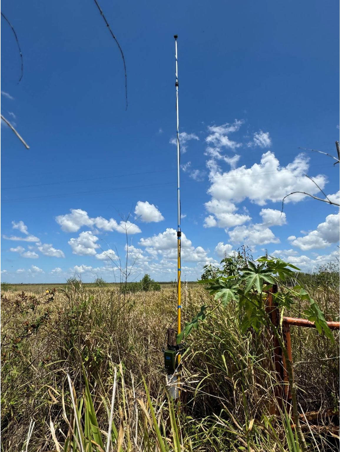
Photograph 5. Photograph looking south at Detector 5 with microphone deployment height of 5.67 meters – Wildlife Acoustics Song Meter SM4BAT FS Ultrasonic Recorder with SMM U2 Ultrasonic Mic.
