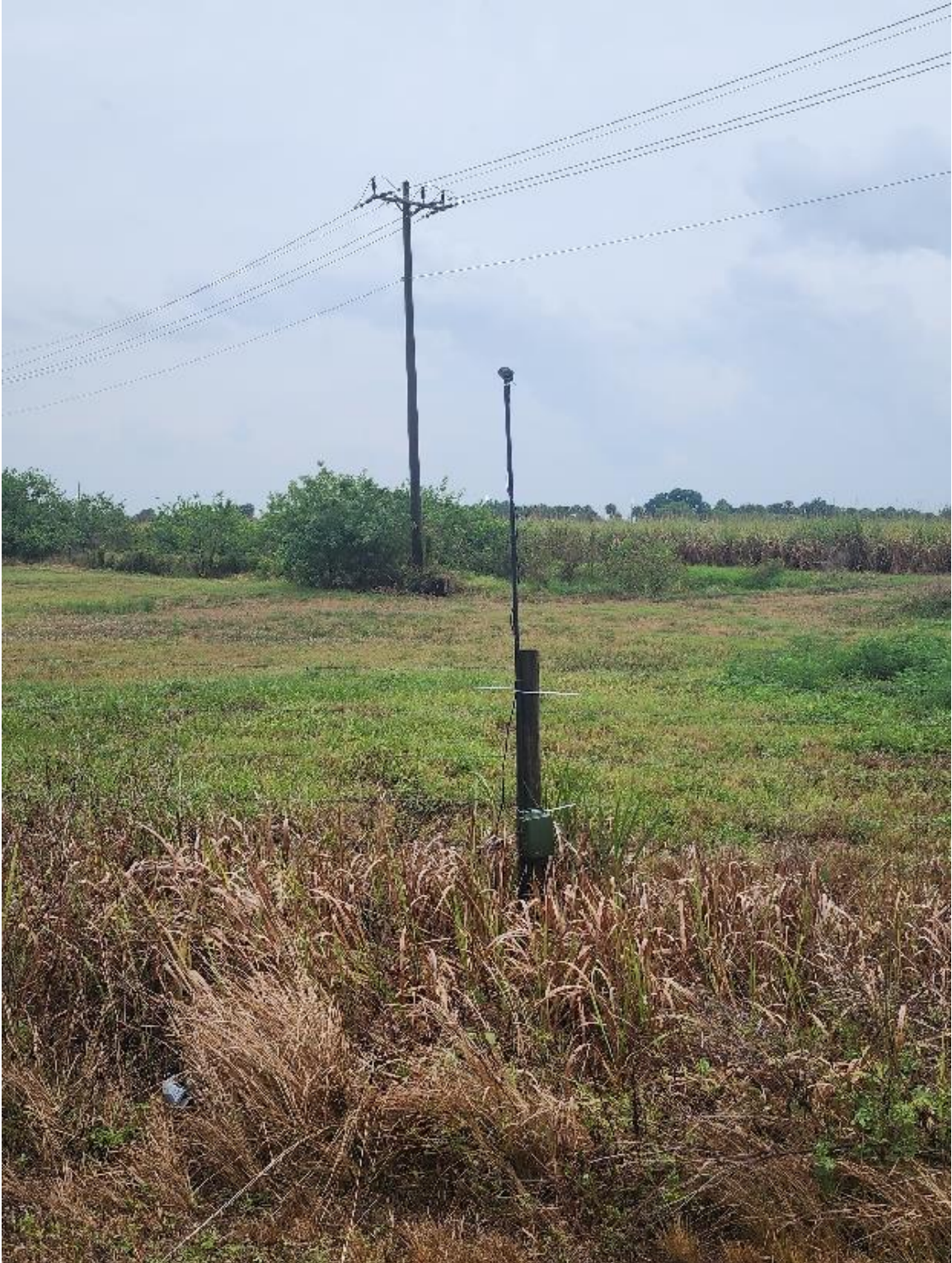
Photograph 15. Photograph looking southeast at Detector 15 with microphone deployment height of 3.04 meters – Wildlife Acoustics Song Meter SM4BAT FS Ultrasonic Recorder with SMM U2 Ultrasonic Mic.
