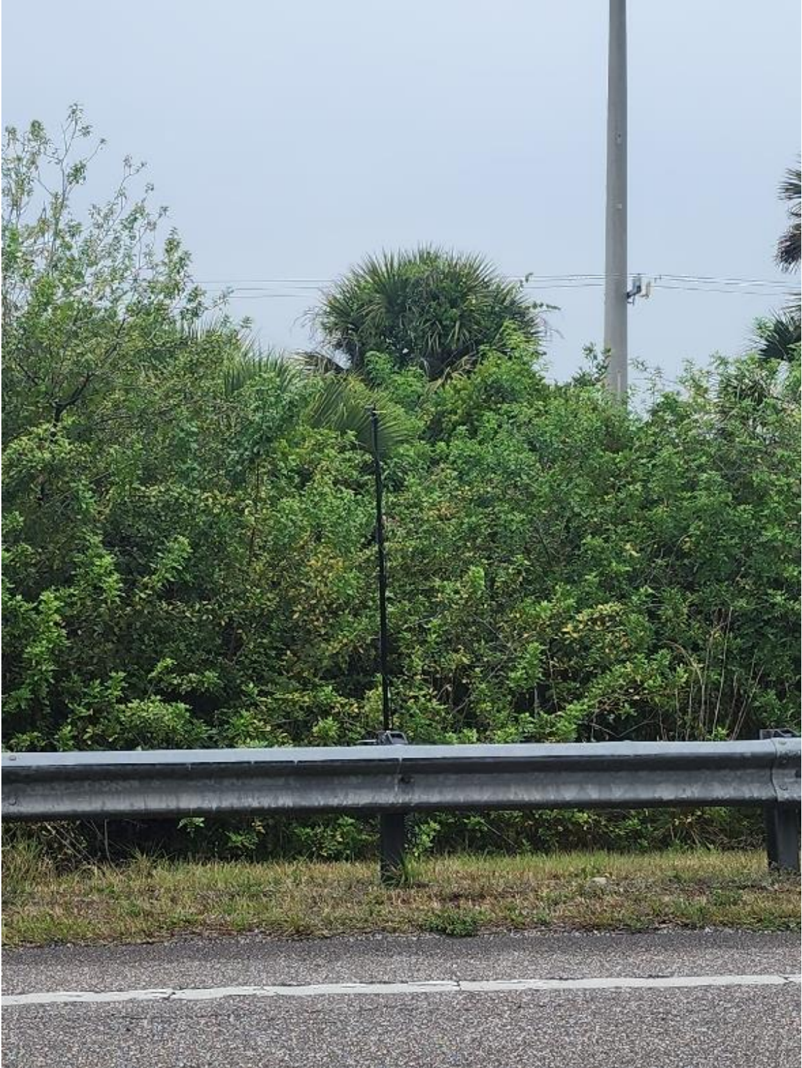
Photograph 12. Photograph looking north at Detector 12 with microphone deployment height of 3.04 meters – Wildlife Acoustics Song Meter SM4BAT FS Ultrasonic Recorder with SMM U2 Ultrasonic Mic.
