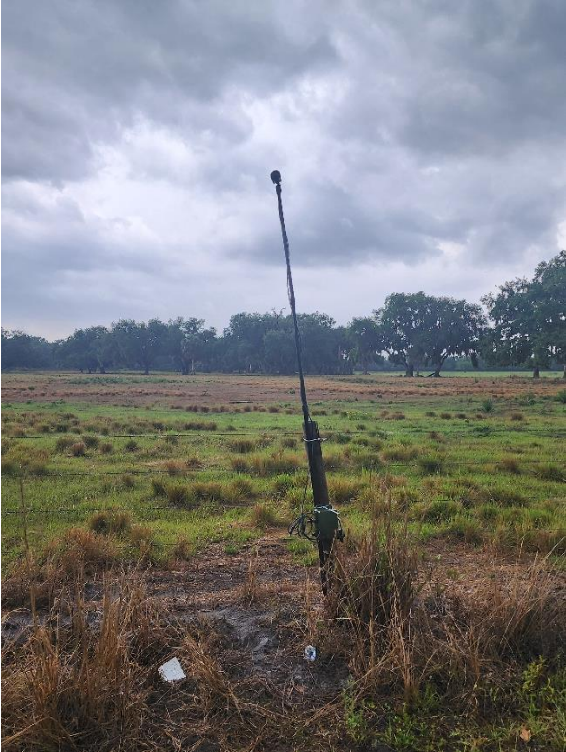
Photograph 17. Photograph looking southeast at Detector 17 with microphone deployment height of 3.04 meters – Wildlife Acoustics Song Meter SM4BAT FS Ultrasonic Recorder with SMM U2 Ultrasonic Mic.
