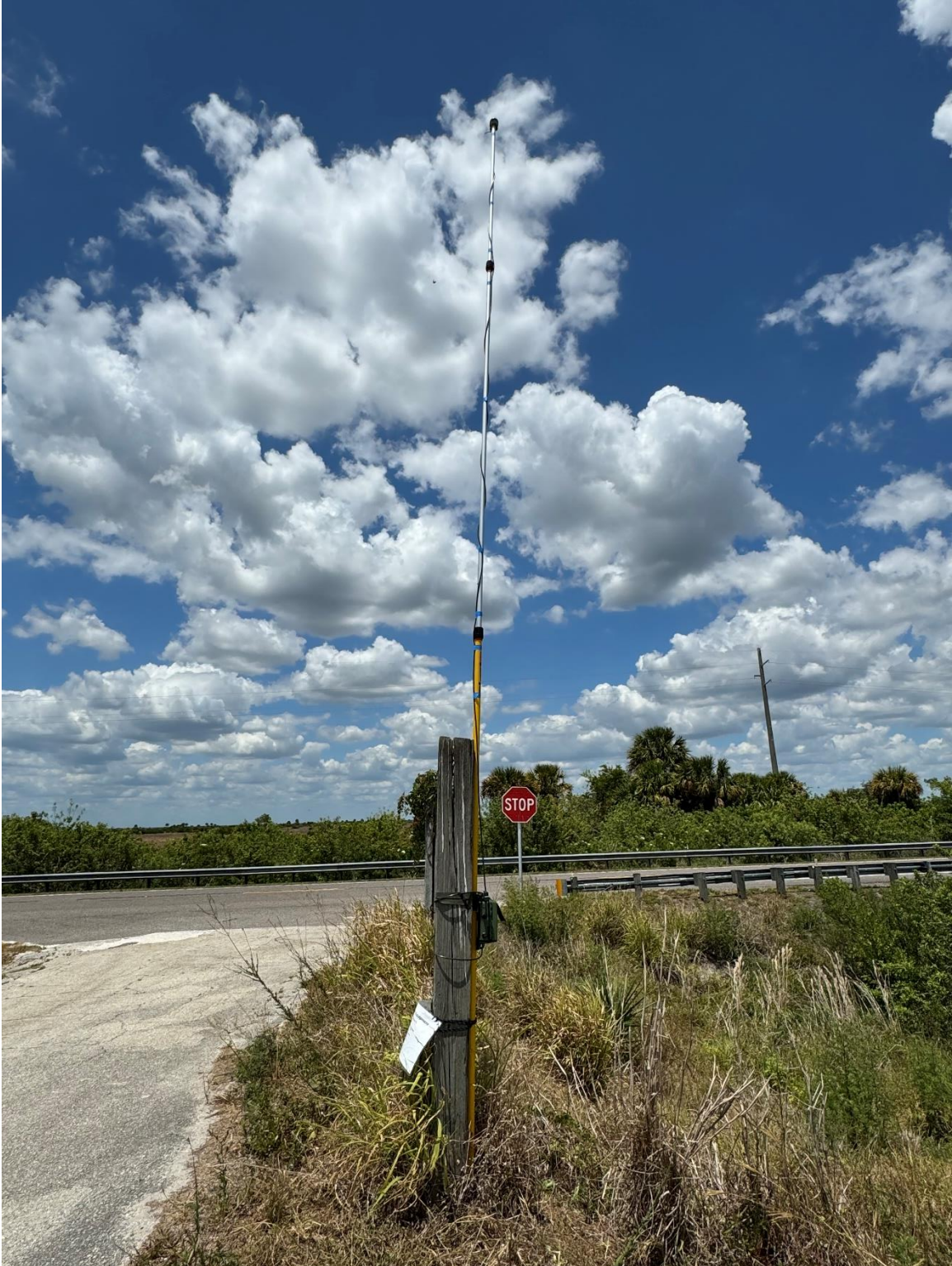
Photograph 7. Photograph looking south at Detector 7 with microphone deployment height of 5.94 meters – Wildlife Acoustics Song Meter SM4BAT FS Ultrasonic Recorder with SMM U2 Ultrasonic Mic.
