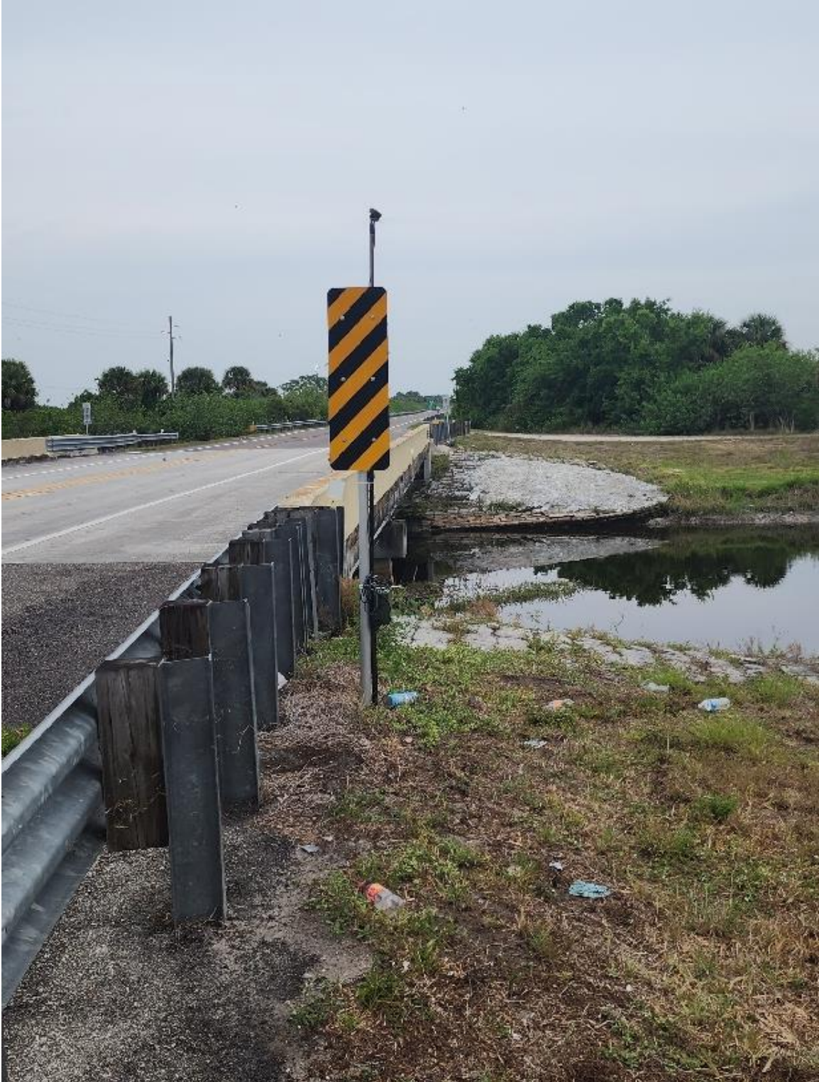
Photograph 9. Photograph looking east at Detector 9 with microphone deployment height of 3.04 meters – Wildlife Acoustics Song Meter SM4BAT FS Ultrasonic Recorder with SMM U2 Ultrasonic Mic.
