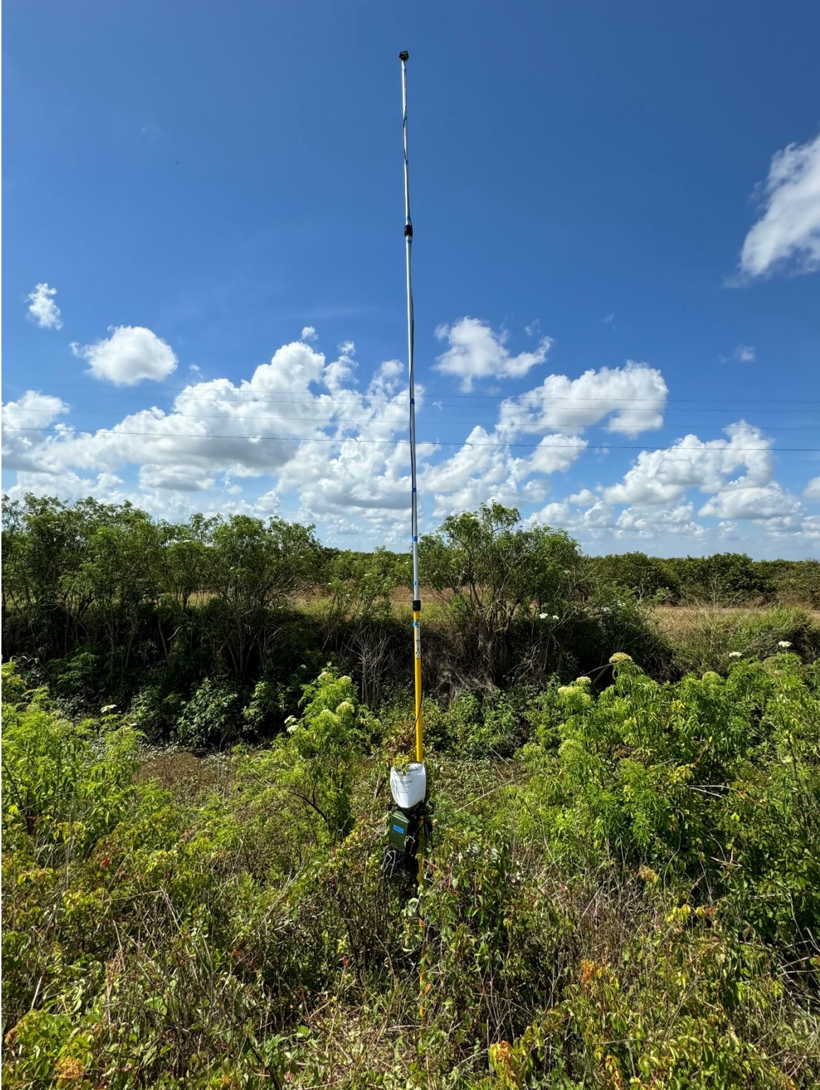
Photograph 3. Photograph looking south at Detector 3 with microphone deployment height of 5.94 meters – Wildlife Acoustics Song Meter SM4BAT FS Ultrasonic Recorder with SMM U2 Ultrasonic Mic.
