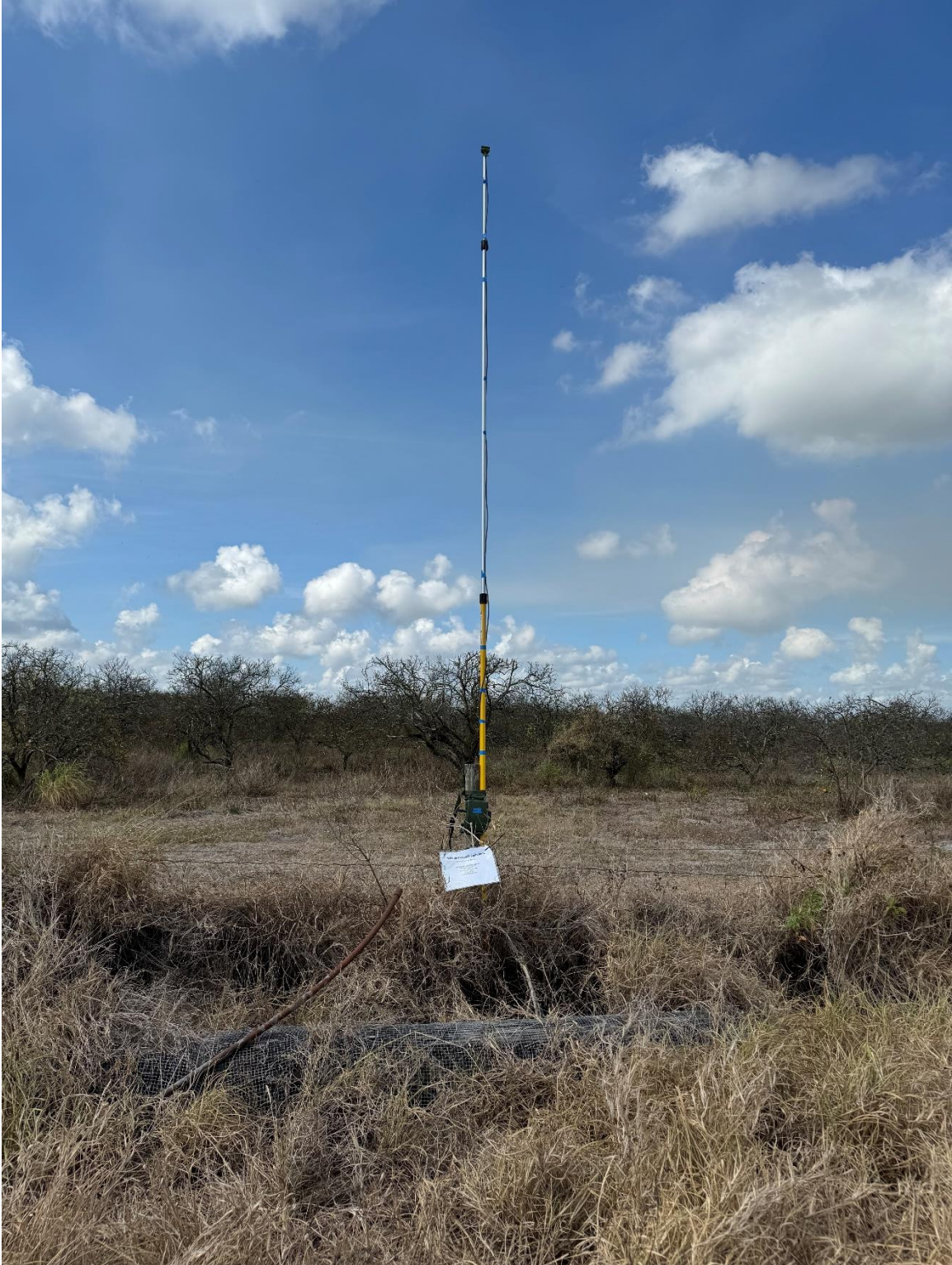
Photograph 2. Photograph looking south at Detector 2 with microphone deployment height of 5.33 meters – Wildlife Acoustics Song Meter SM4BAT FS Ultrasonic Recorder with SMM U2 Ultrasonic Mic.
