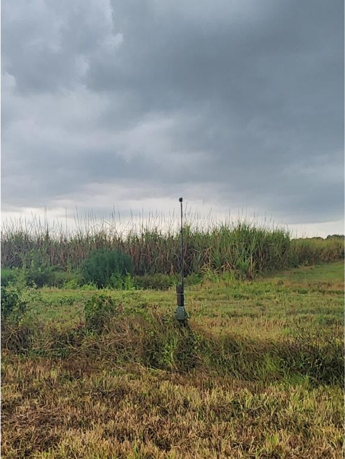
Photograph 16. Photograph looking west at Detector 16 with microphone deployment height of 3.04 meters – Wildlife Acoustics Song Meter SM4BAT FS Ultrasonic Recorder with SMM U2 Ultrasonic Mic.
