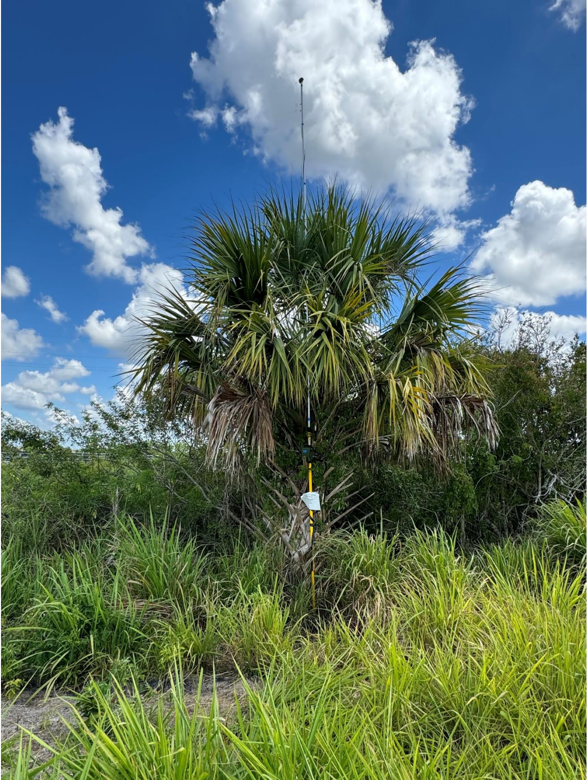
Photograph 4. Photograph looking south at Detector 4 with microphone deployment height of 6.86 meters – Wildlife Acoustics Song Meter SM4BAT FS Ultrasonic Recorder with SMM U2 Ultrasonic Mic.
