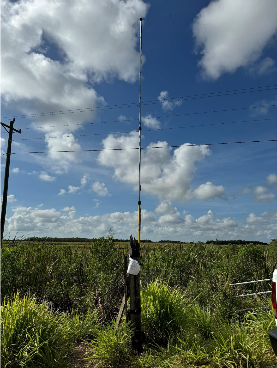
Photograph 1. Photograph looking south at Detector 1 with microphone deployment height of 5.94 meters – Wildlife Acoustics Song Meter SM4BAT FS Ultrasonic Recorder with SMM U2 Ultrasonic Mic.
