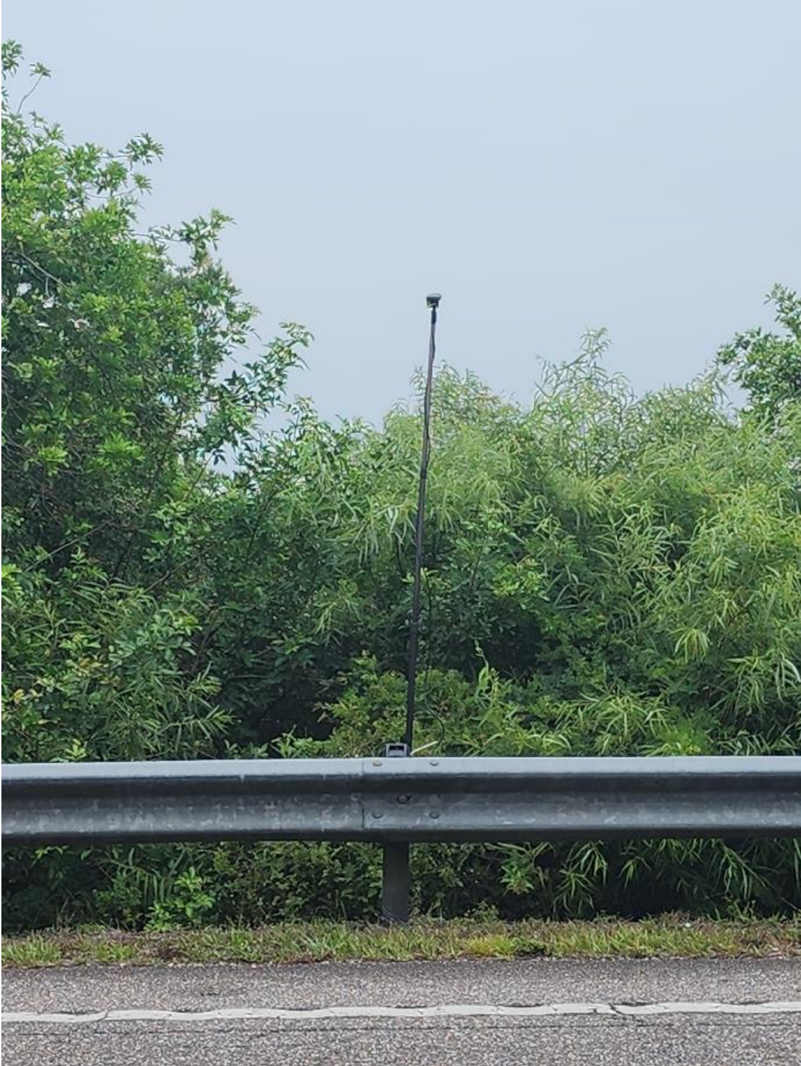
Photograph 13. Photograph looking southeast at Detector 13 with microphone deployment height of 3.04 meters – Wildlife Acoustics Song Meter SM4BAT FS Ultrasonic Recorder with SMM U2 Ultrasonic Mic.
