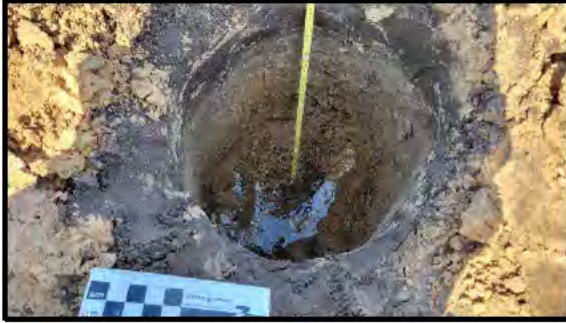
Photo 5.1. Stratigraphy within fallow sugarcane fields adjacent the south side of SR 70, facing west. Note the water intrusion at the bottom.
