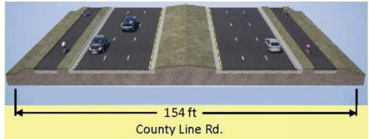
County Line Road proposed six-lane typical section consists of three-lanes in each direction (36 ft wide) separated by a 30 ft median with 10 ft shared use paths on both sides.
