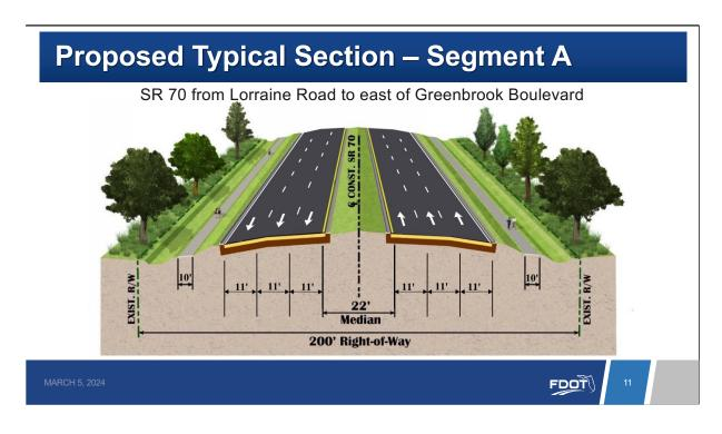
Segment A will be widened to a 6-lane divided highway with 11-foot travel lanes, a 22' median, curb and gutter on the inside and outside of the roadway, and 10-foot shared used paths. Other improvements include drainage system enhancements and lighting.
