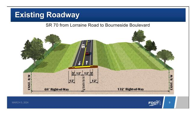
This section of State Road 70 is a 3.1 mile 2-lane undivided rural principal arterial highway with 12-foot travel lanes. The current conditions do not include pedestrian access or lighting through the corridor.
