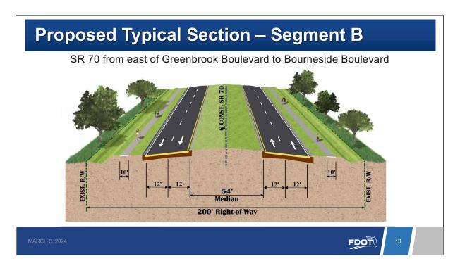
Segment B will be widened to a 4-lane divided highway with 12-foot travel lanes and a 54-foot median. This segment will also include curb and gutter on the inside and outside of the roadway and 10-foot shared use paths. Other improvements include construction of four bridges over Braden River crossings, drainage system enhancements, the construction of two ponds, and lighting.
