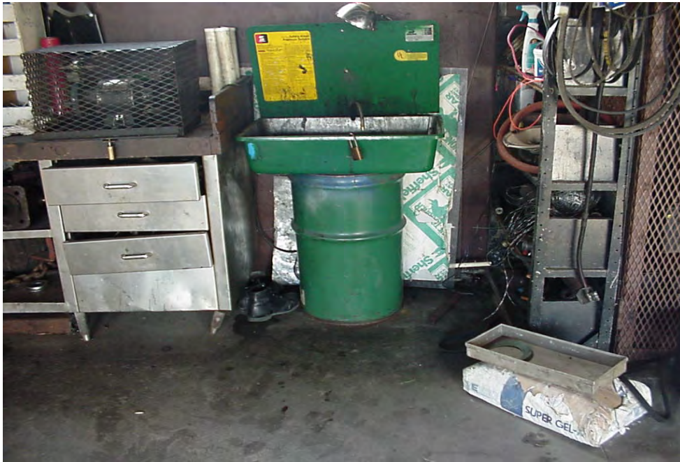
Photo 22. AOI 10: Parts cleaning sink and concrete staining
