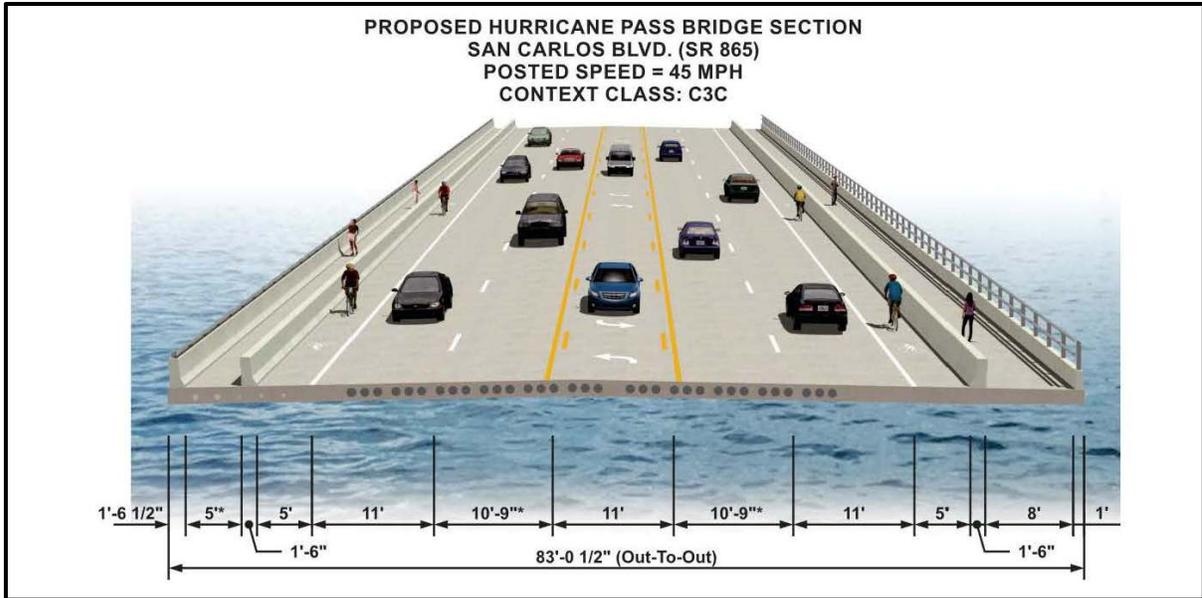
**Figure 1.4.** Typical Section of the proposed Hurricane Pass Bridge improvements.
