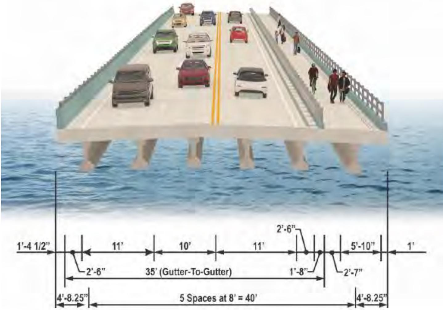
Figure 1-3. Typical Section of the SR 865 (San Carlos Boulevard) improvements from Main Street north to Hurricane Pass Bridge
