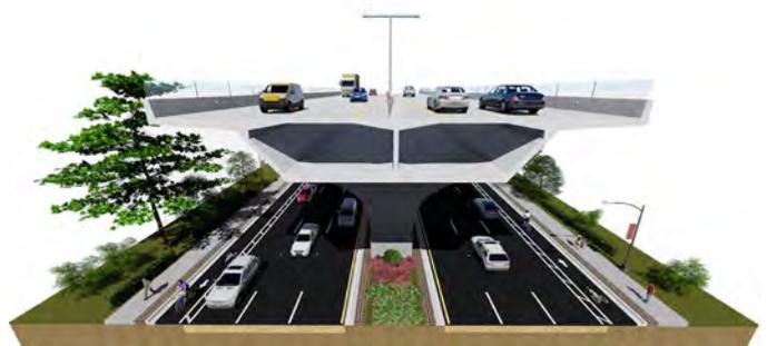
Figure 41: Alternative AB – Elevated Throughway Typical Section - North of the Manatee River
