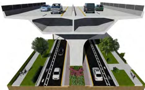
Figure 49: Alternative D – Elevated Throughway Typical Section
