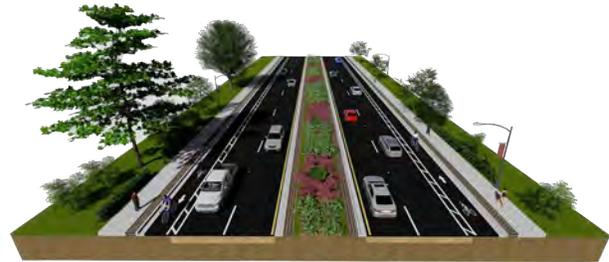
Figure 50: Alternative D – At-Grade Widening Typical Section
