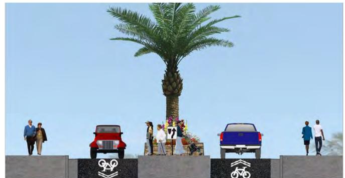
12' Sidewalk and Curb/Gutter | 11' Travel Lane | 12' Median/Turn Lane | 11' Travel Lane | 12' Sidewalk and Curb/Gutter
