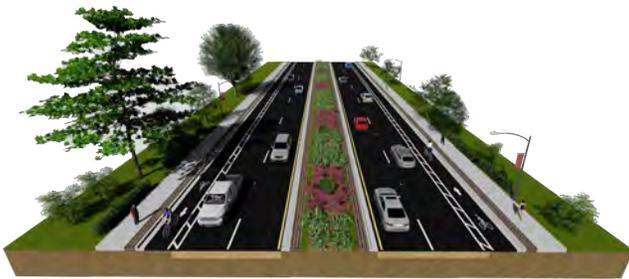
Figure 42: Alternative AB – At-Grade Widening Typical Section
