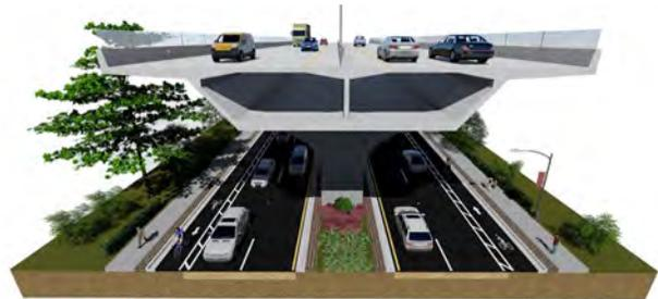
Figure 43: Alternative B – Elevated Throughway Typical Section: South of Manatee Avenue
