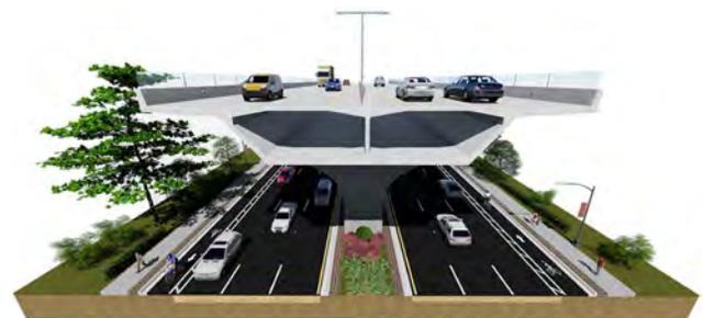
*Elevated Throughway Typical Section: Six Lanes at Local Level*
