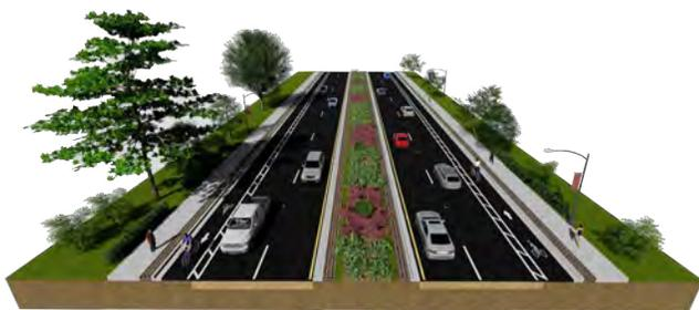
Figure 46: Alternative B – At-Grade Widening Typical Section
