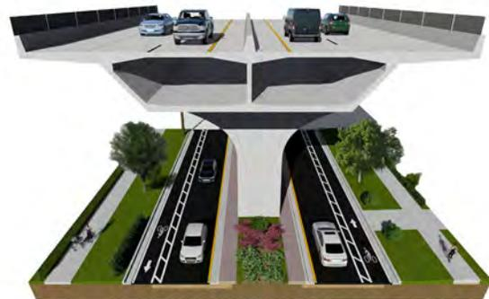
*Elevated Throughway Typical Section: Two Lanes at Local Level*
