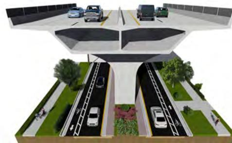
Figure 44: Alternative B – Elevated Throughway Typical Section: North of Manatee Avenue
