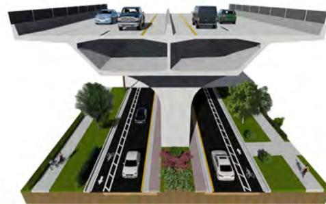
Figure 47: Alternative C – Elevated Throughway Typical Section
