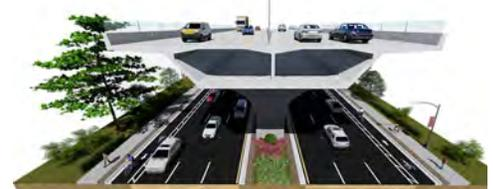
Figure 34 Alternative A – Elevated Throughway Typical Section
