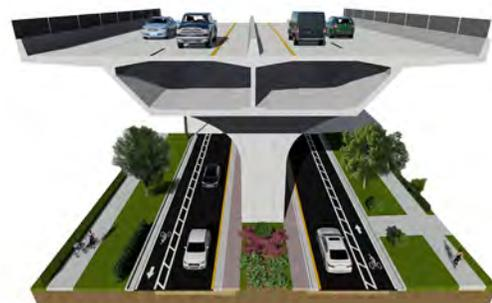
Figure 40: Alternative AB – Elevated Throughway Typical Section - Between the Manatee River & Manatee Avenue
