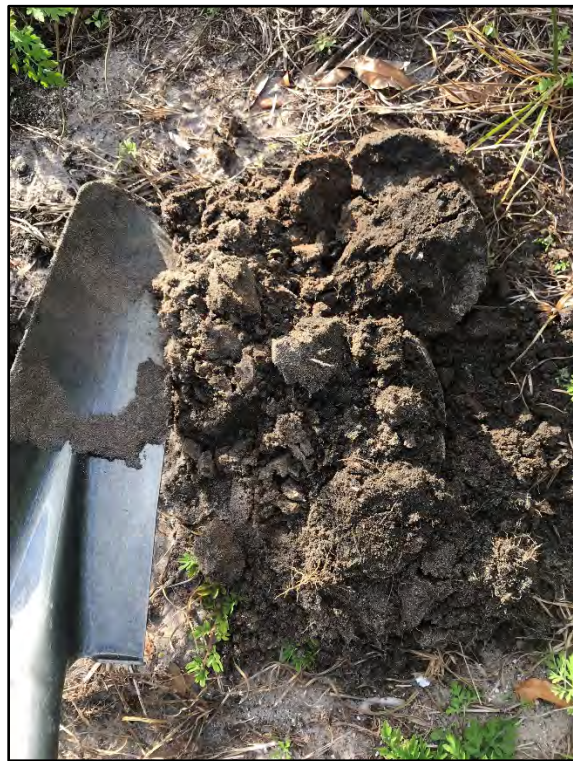
Soil sample #2 – fill material observed within sample.
